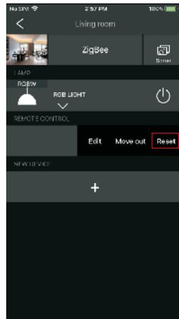
From your ZigBee controller or hub interface, choose to delete or reset the remote as instructed, indicator flashes 3 times quickly to indicate successful removing.
