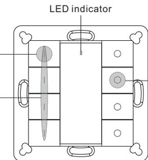
**Step 1:** Press and hold down until LED indicator turns on.
