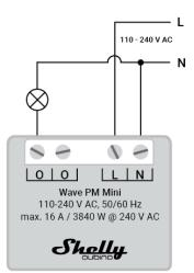
LEGEND Device terminals: N: Neutral terminal L: Live terminal (110-240 V AC) O: Load circuit output terminal (bridged internally) Wires: N: Neutral wire L: Live wire (110-240 V AC)
