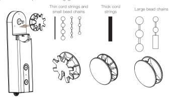
Semove the teeth where from the cord or chains come out on cover plate; then lock the cover up
