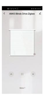
7.this page can operate the motor going UP, STOP, DOWN; click 'More' to get into multiple functions setting page
