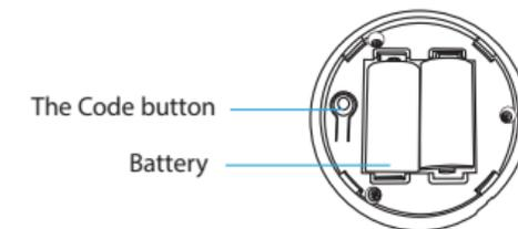
**Notice:** Please use USB power supply, the backup battery can only work for two days. Plug in the USB power supply and load the battery at the same time, then the sensor will work in priority.
