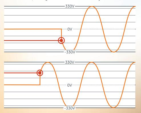
ZeroX Detection technology guarantees that our devices switch on/off close to 0V, thereby minimizing wear and tear on the relay and significantly extending its lifespan.
