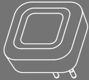
1. Insert the siren with the plug into an outlet.
