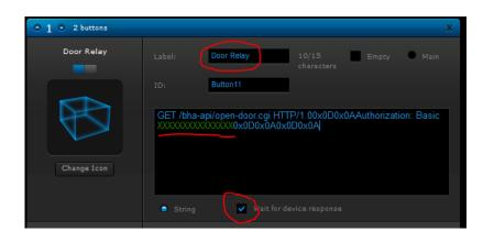
You can use the door opener and the IR LED function after you have entered the authentication details for "Door Relay" and "IR LED" saved them.
