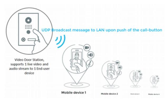
The mobile devices (e.g. smartphone, tablet, smart-home panel) listen for UDP Broadcast messages within the LAN from the door station. If a valid UDP Broadcast message (valid: fits to the call-button number) is received from the door station by the mobile devices, then the mobile devices play a "ding-dong" notification sound and offer the End-user the possibility to take the call upon user-interaction by e.g. pressing a button on the mobile devices.
